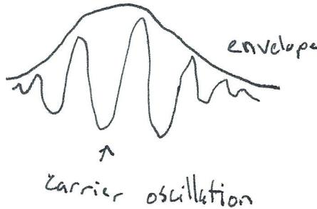
$$\text{Group velocity } \vec{v}_g = \frac{d\omega}{d\vec{k}} \quad \omega = \omega(\vec{k})$$
